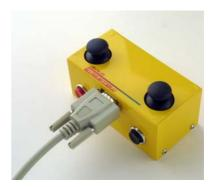
The Meccanisms Director connects to the Sensor Expansion Port and provides two XY Joysticks and Four Control Buttons, to give you manual control over the most complex models, particularly cranes.
